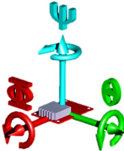
Figure 3.10: 3D analyses of orientation finding using accelerometers.
