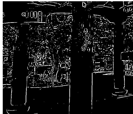
(d) Thresholded result of Difference of Gaussians.
